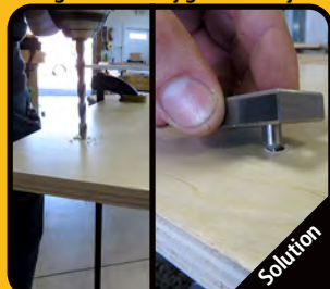
Drill 1/4" hole, slide in slot, and drill
